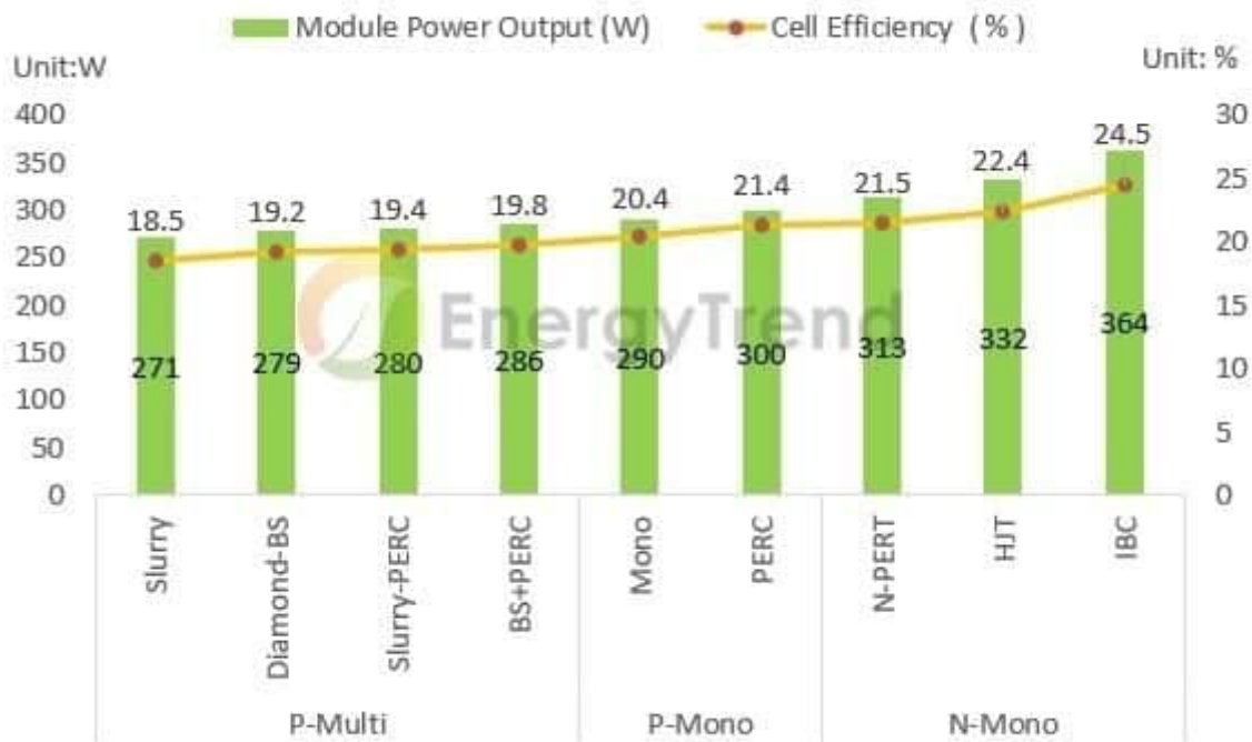
Figure: Cell Efficiency (%) and Module Power Output (W) By Different Types
